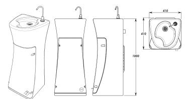
INLET: 860mm ABOVE BASE 100mm LEFT OF CENTRE LINE (from back) OUTLET: 860mm ABOVE BASE 30mm LEFT OF CENTRE LINE (from back)
